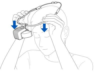
4. Pull the frame strap's sliders left and right to fit your b.g. to your head.
