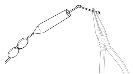
4. Use the longnose pliers' cutter to cut off the excess wire at the knot.
