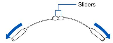
2. Pull the silicone parts of the frame strap, moving them toward the sliders.
